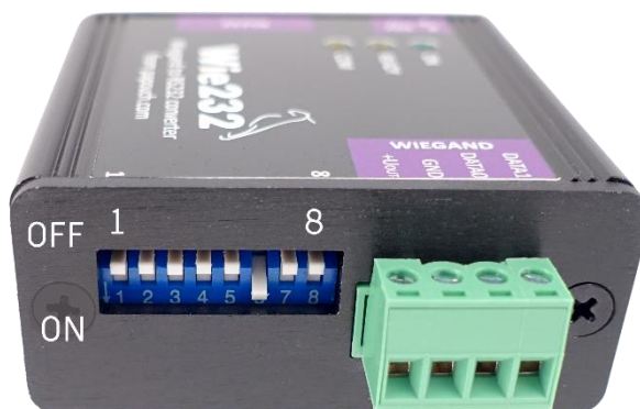
Fig. 2 - configuration switch position and ON / OFF positions
