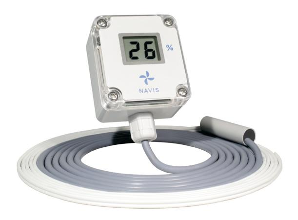
LEVELWATCH C1 is basic, battery operated water level monitor. It continuously measure and display water level with one percent resolution. Capacitance operating principle, without moving parts, ensure long life time and maintenance-free operation. LW C1 is
