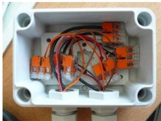
4. Connect the wires with the Wago clamps. Write down which color of the extension cable is V+, V-, Data+, Data- and cable shield. Pay attention that the plastic collar of the wire end ferrule is not clamped and can be fully seen at the backside of the Wago clamp.
