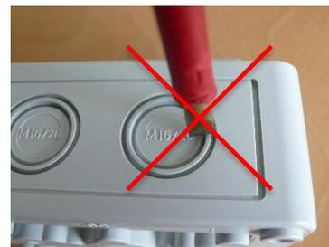
2. Place the cable glands into the holes and tighten the nut properly. Make sure the nut is placed with the flat side to the housing.
