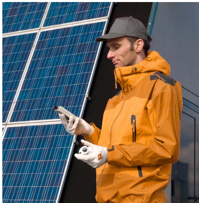
Figure 1 Pyranometer in use with LI19 read-out unit.
