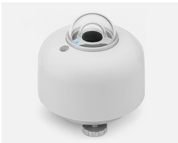
Figure 2 Example of a Hukx spectrally flat Class A pyranometer, SR300-D1. This model is recommended for PV system performance monitoring as well as research-grade diffuse radiation measurement. Digital output via Modbus RTU over RS-485.
