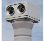
Using so called backward-scattering technique it measures the amount of particles in the air that limit the visibility. It emits pulses of infrared light and measures the intensity of the backward-scattered light of the suspended particles in the atmosphere, using suitable algorithms to convert the measurements to meteorological visibility values.
