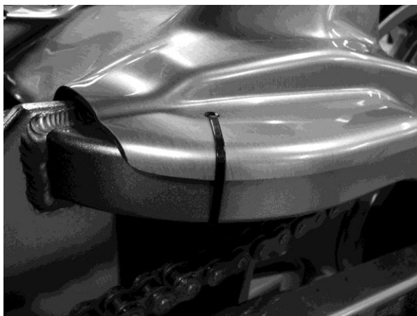
Position of cable tie
