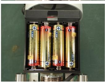
Close the battery cover and then slide back the upper housing case until it locks into place.
