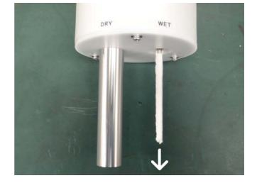
Place a new wick over the sensor and put the ventilation tube back in place.
