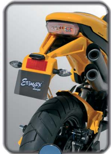
Plate holder cover in ABS for original plate holder Tail light white LED
