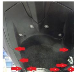
8 plastic rivets location
