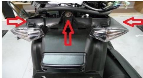
Location of the screws securing the mudguard
