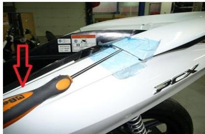
Tip to unclip the cover : use a small flat screwdriver to act as a lever in the direction of the arrow, while taking care to protect the cover.
