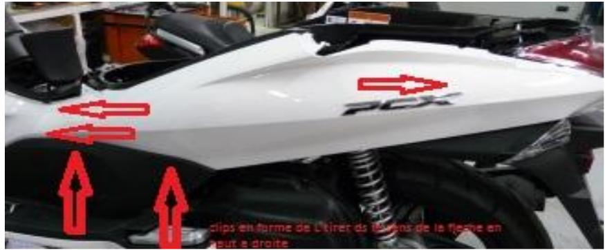
Clips' location : pull in the direction of the arrow at the right top to exit the fairing
