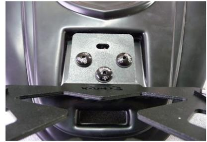
Washers, Nylock nuts and screw 5x25 small head's location.
