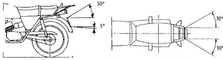
Width of number plate location: 280 mm - Height of location : 210 mm
