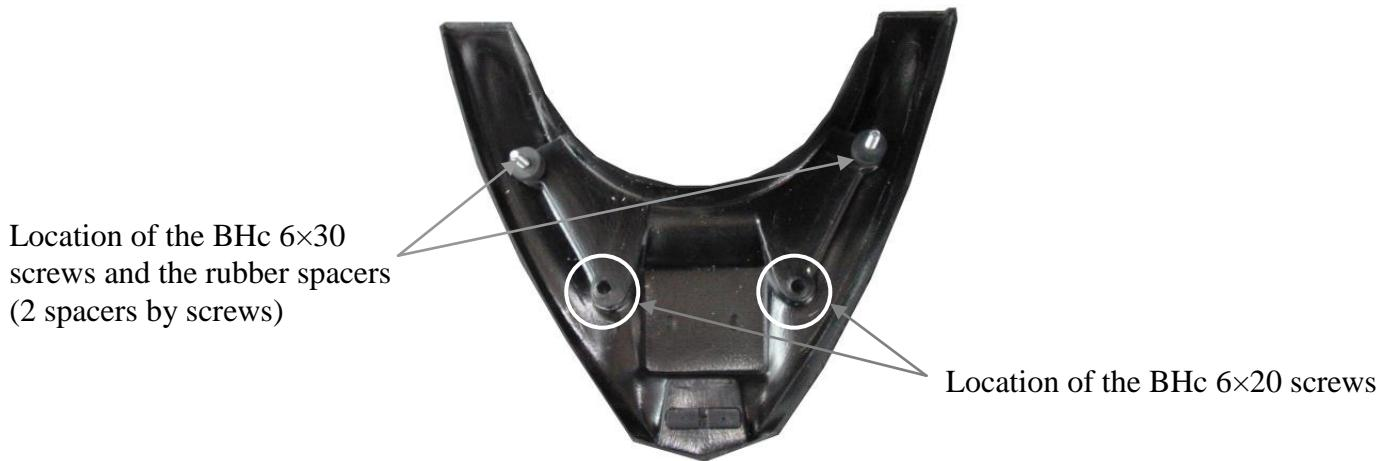
Location of the BHc 6×30 screws and the rubber spacers (2 spacers by screws)
