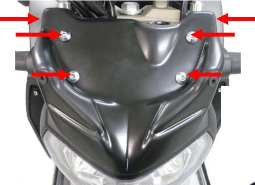
Whole holed screw + ring + steel washer Ø8 + blind nut.
